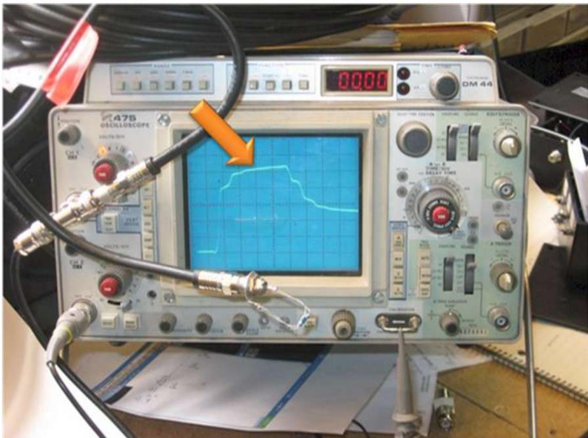
A pair of 75 ohm resistors were added in parallel as a termination on the cable. This of course terminates the cable in 37.5 ohms which shows a severe mismatch compared to the cable terminated with the 75 ohm proper termination.
