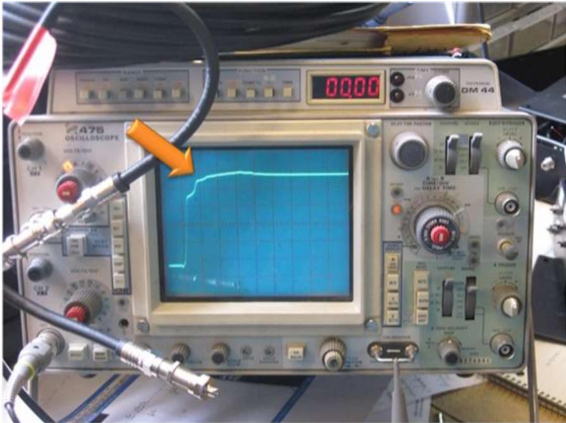
A 75 ohm terminator was added to the end of the 75 ohm cable and the reflection was nearly eliminated.
