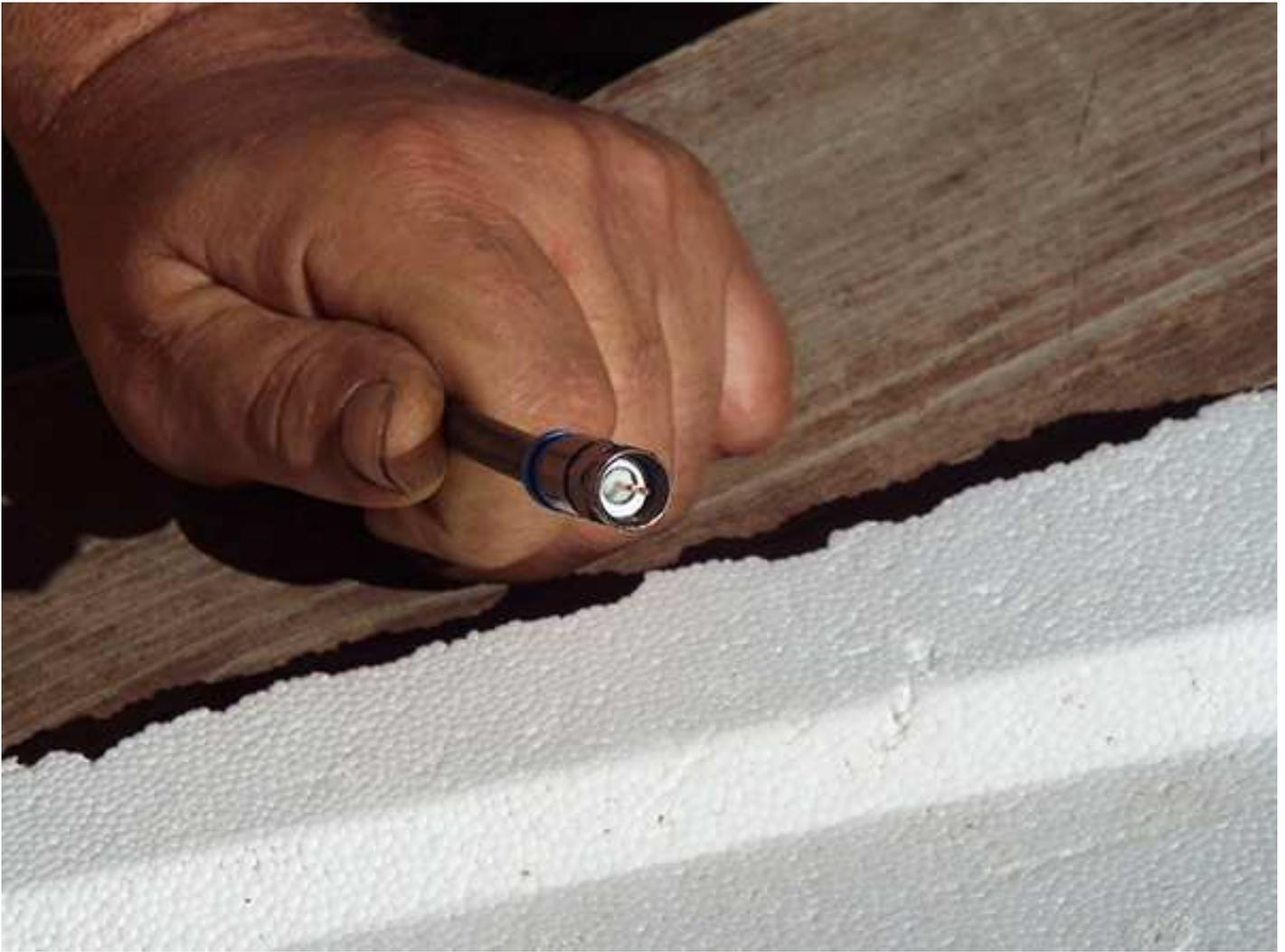
Carefully make sure that no small wires can cause possible shorting and that the center insulator is flush with the connector bottom as shown.
