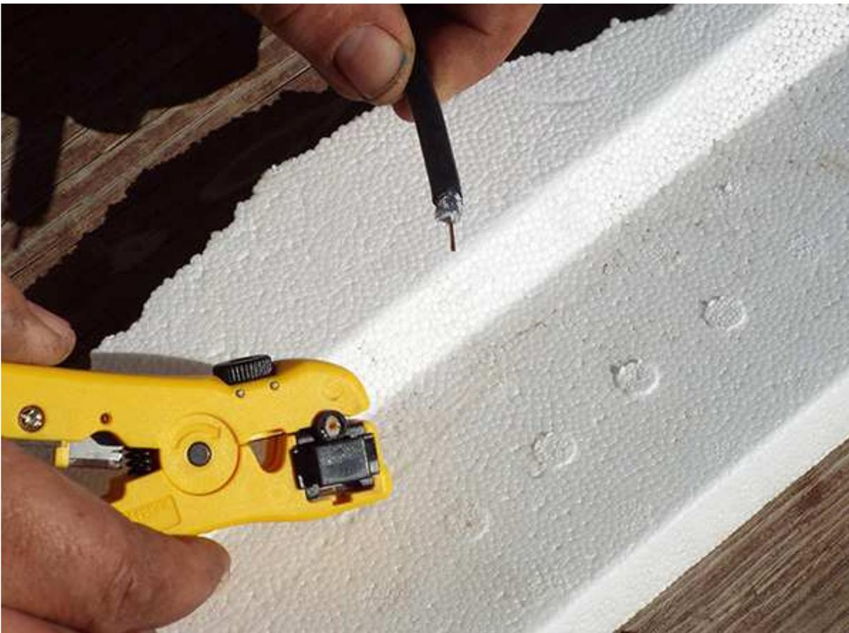
Pull the tool away exposing the trimmed cable end.
