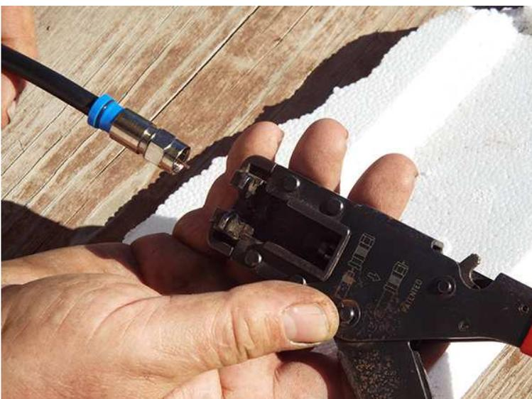
With the compression tool open as shown prepare to insert the cable.
