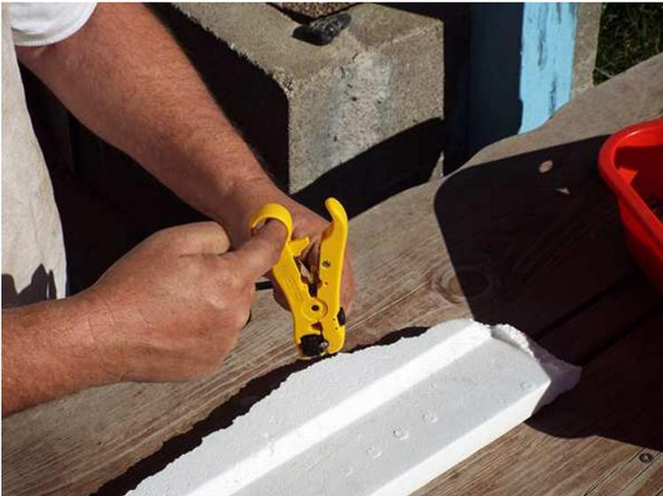
Twirl the tool several rotations until it turns easily and begins to slide off the end with a gentle tug. Do not let your finger slip out of the loop into the blade!
