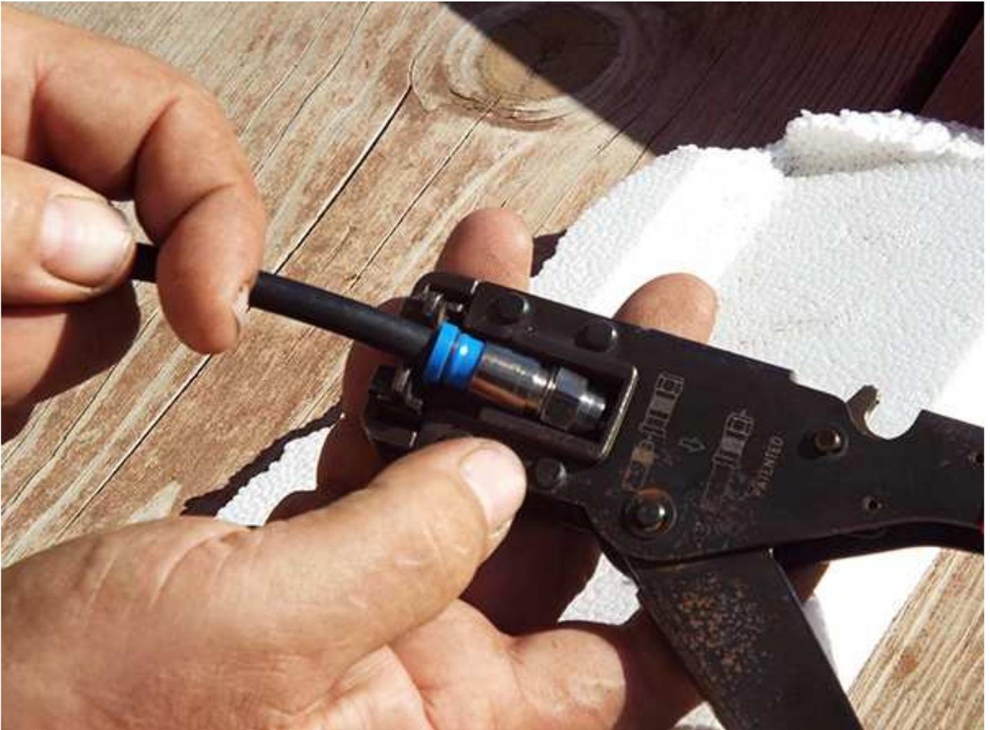
Angle the connector into the tool while inserting the center conductor into the hole provided.
