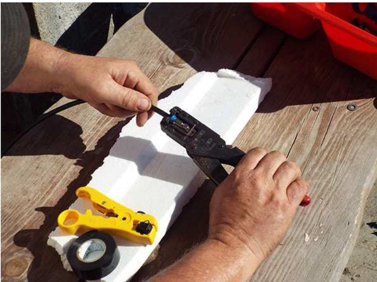
Begin squeezing the handle to press the blue sleeve into the connector shell.
