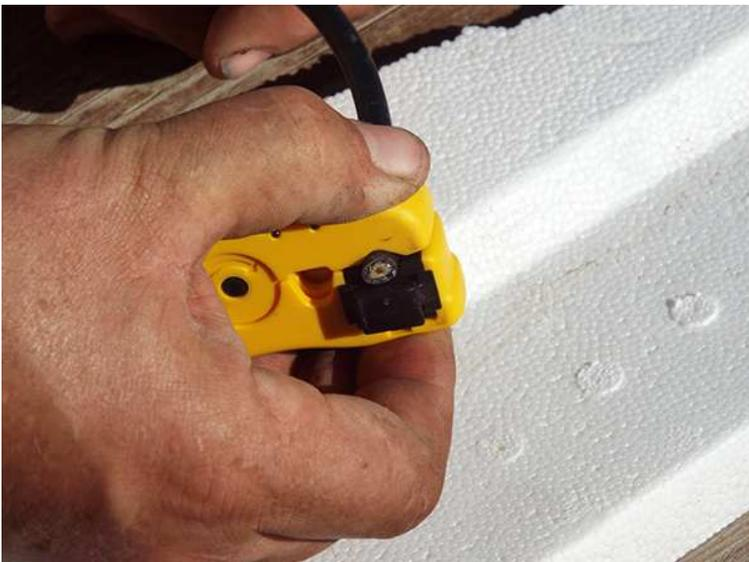
Clamp down the tool with fingers as shown to break through the insulation.
