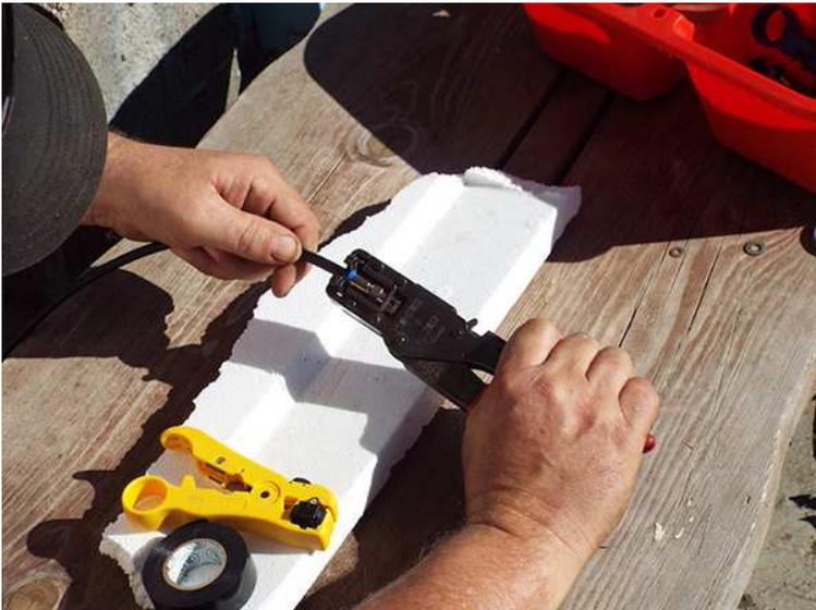
Squeeze the handles firmly which will snap and release the ratcheting handle.
