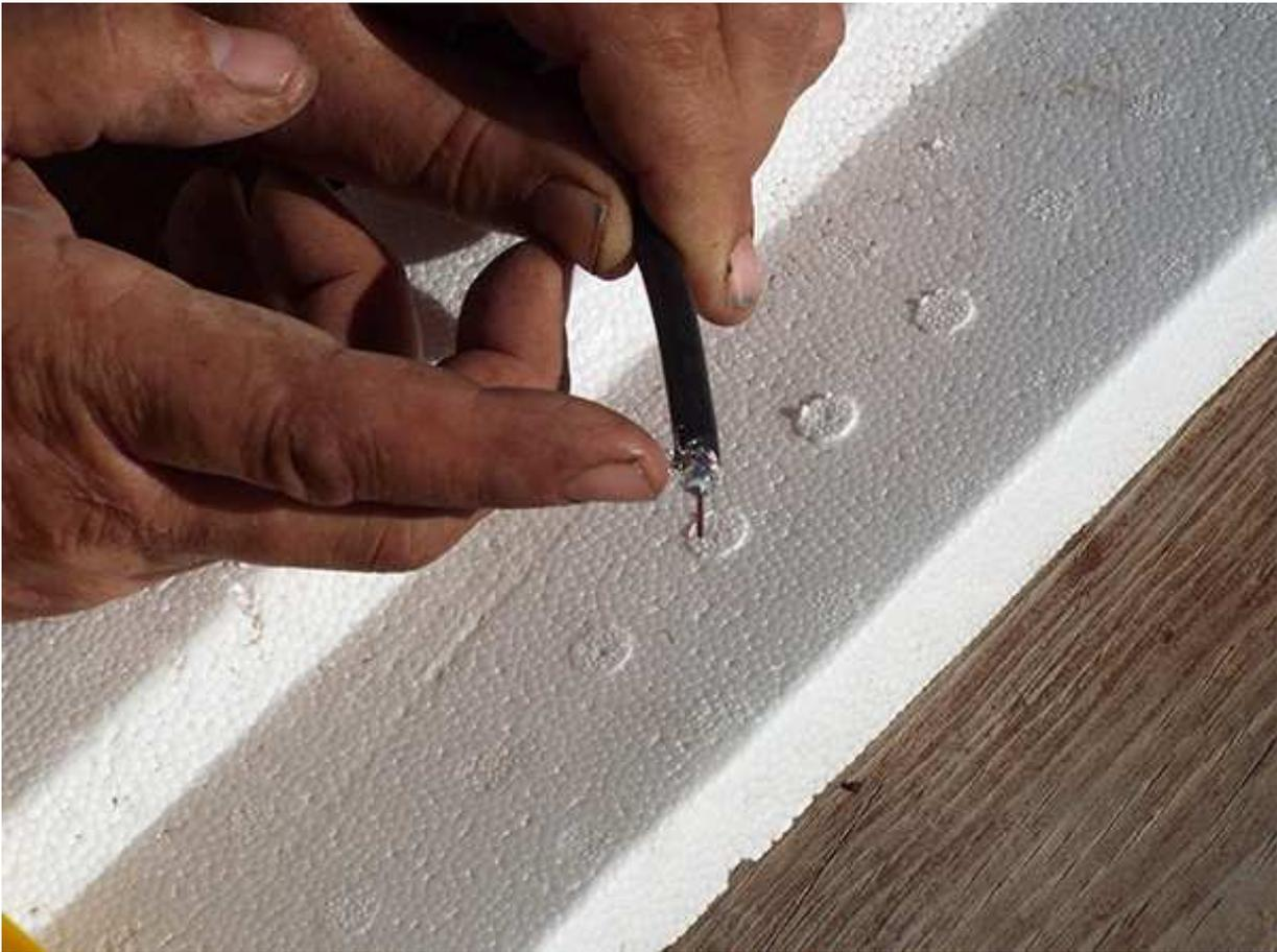
Fold back the braid only onto the outside insulation.
