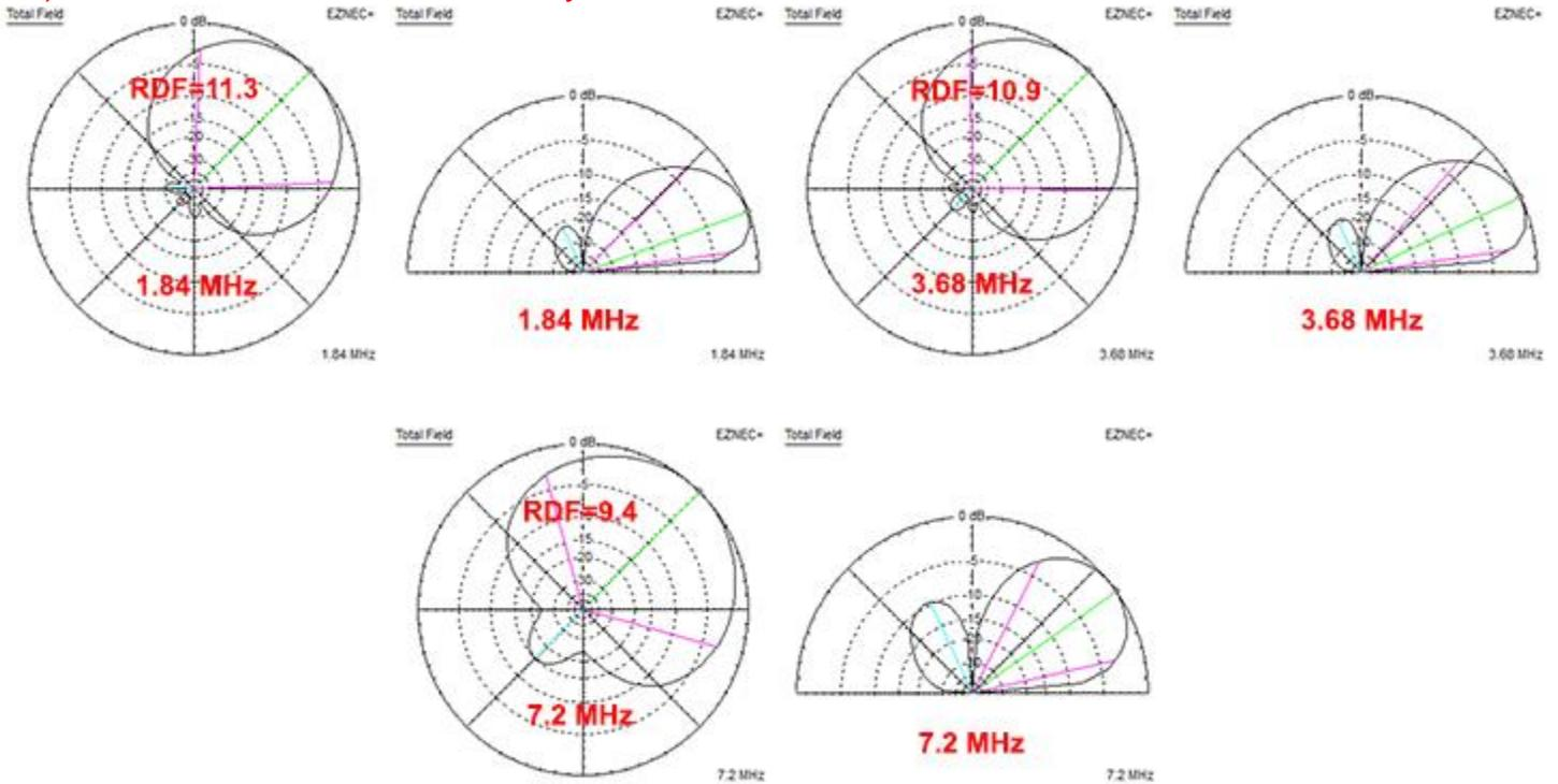
**85 Foot Diameter.** One customer adjusted pair of delay cables of 40 degrees for the long delay cable and 20 degrees for the short delay at 1.84 MHz (Max RDF mode) with customer modified delay cables.
