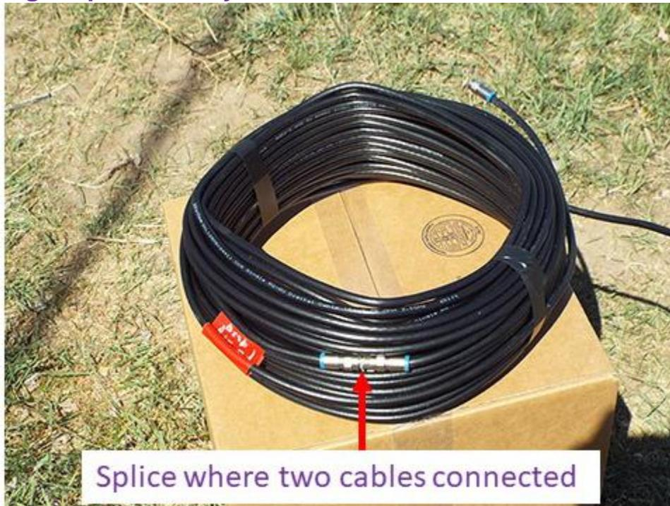
Splice where two cables connected
