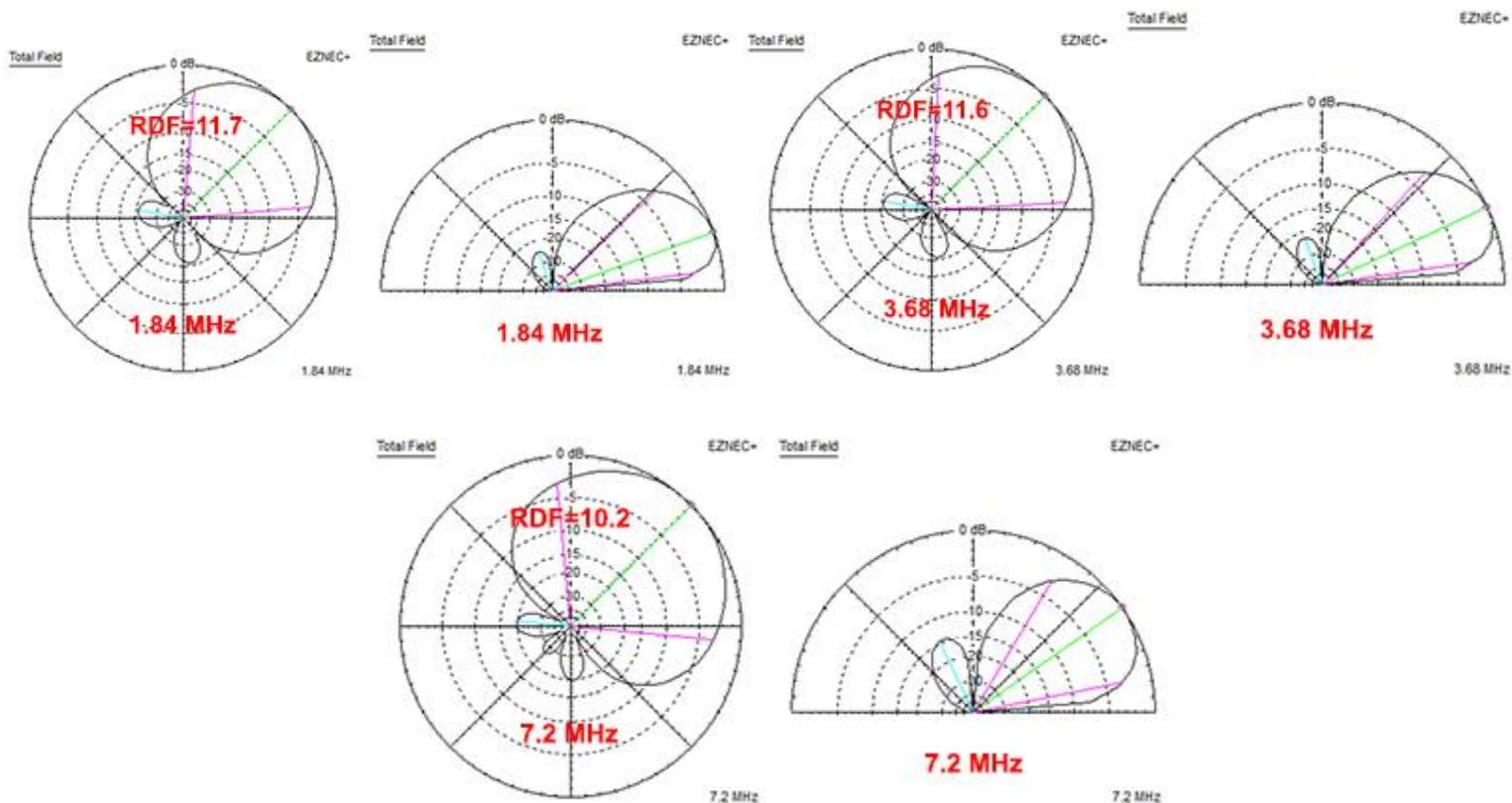
**85 Foot Diameter.** One customer adjusted pair of delay cables of 70 degrees for the long delay cable and 35 degrees for the short delay cable at 1.84 MHz (Max Front to Back mode) with customer modified delay cables.
