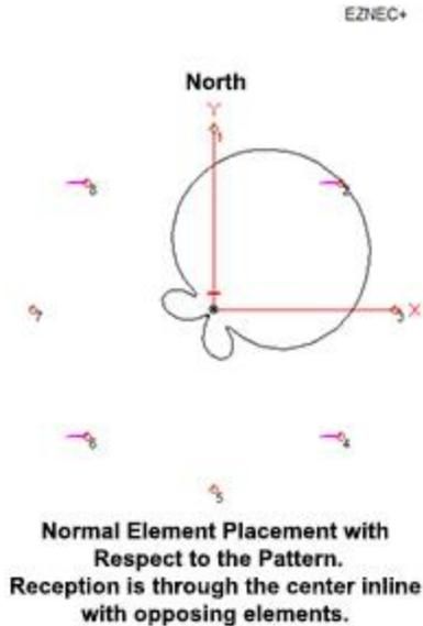
The receiving elements can be placed at 85 or 113 foot diameter depending on the user's needs. The elements are placed in a octagon configuration. The elements need to maintain their equidistant symmetry. The array can be directionally offset if necessary. The HIZ-SS2 and HIZ-SS2-Plus Shack Switch controls can accept offset values and provide a readout of actual direction.
