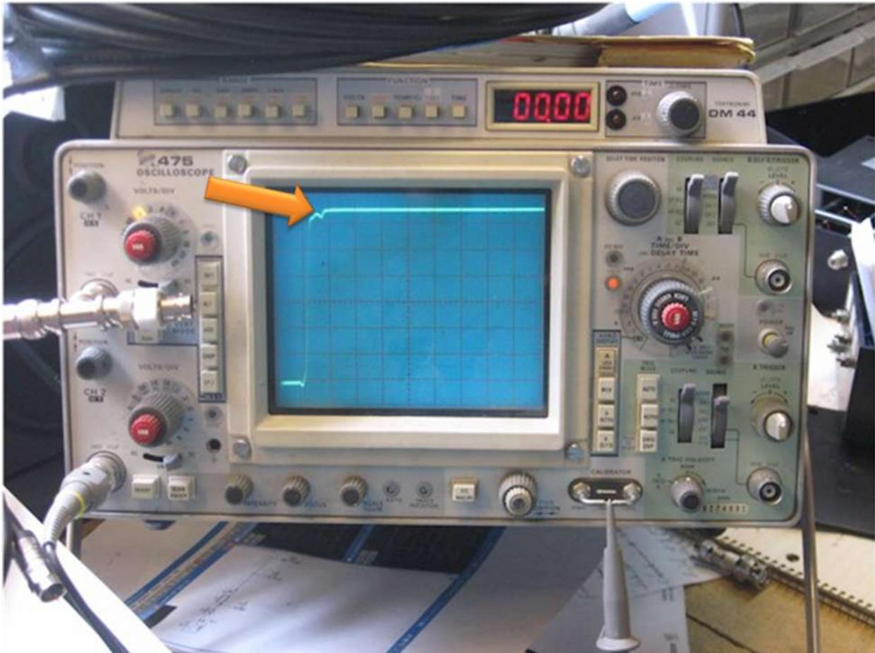
This picture shows the trace produced by connecting the A Gate output on the back of the scope into the A vertical input on the scope. This was done with a 50 ohm coax cable and a 50 ohm terminator. Notice the little wiggle of the trace at the beginning of the top part. This is showing a slight reflection on the connecting cable. **Put scope settings here. (time, vertical)**
