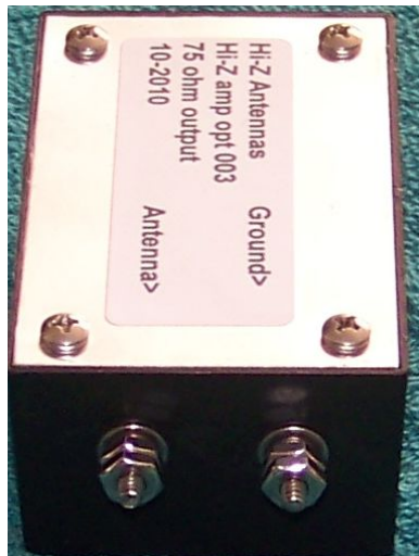
Terminals to Ground and Vertical
