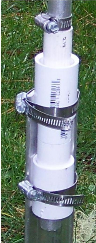
Holding clamp. Clamp so that the lower Vertical end is exposed to connect Hi-Z Amp, no more.
